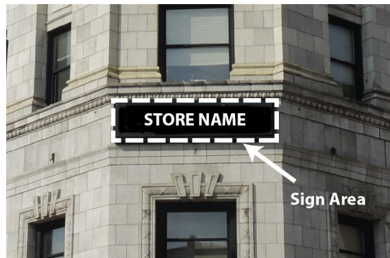
Figure M: Illustration of computing the sign area for wall signs with a background panel or cabinet.
